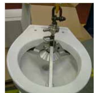
Two different types of clamping tools used with to lift ceramic toilet seats.
