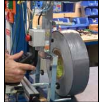
Roll handling pneumatic gripper, paper roll with adjustable joystick control
